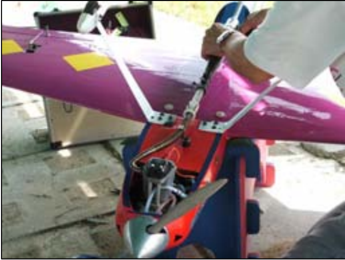
Photo left: Serious pattern plane power: YS 1.40 fuel injected with tuned pipe (Fashion pattern plane).
